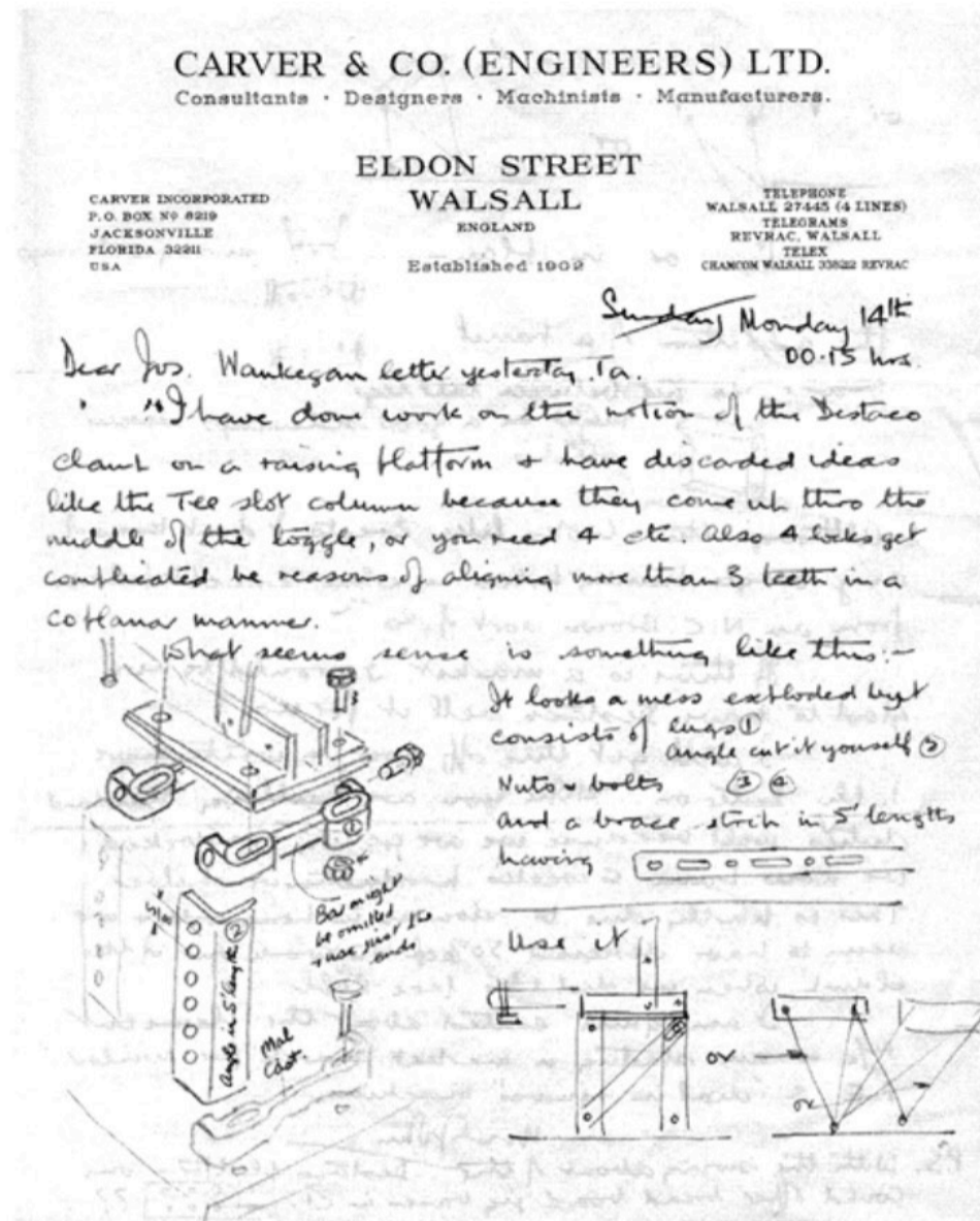
John Carver's inventive mind was never still and this letter to his brother, Jos, who was travelling in the United States, shows his facility for design, both in words and pictures, in this instance for a variant of the Carver clamp
